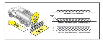
Try to achieve a triple overlap. A double overlap can work too, but triple is the most common and a little more forgiving. A triple overlap ensures uniform placement of material, and that's what we want.
